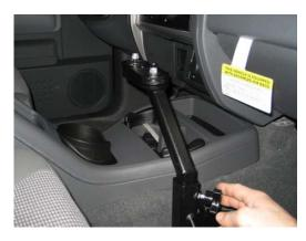
Insert inner telescoping pole assembly and thread lock handle into pole support base assembly.
